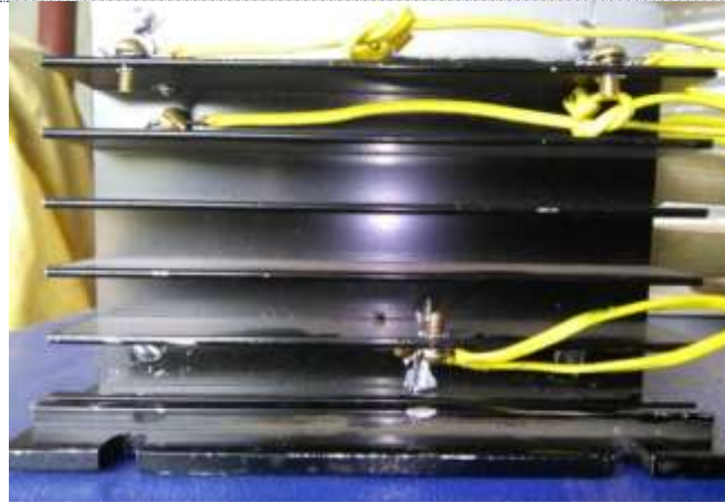
Fig. 1 Thermocouple Connection on Fin
